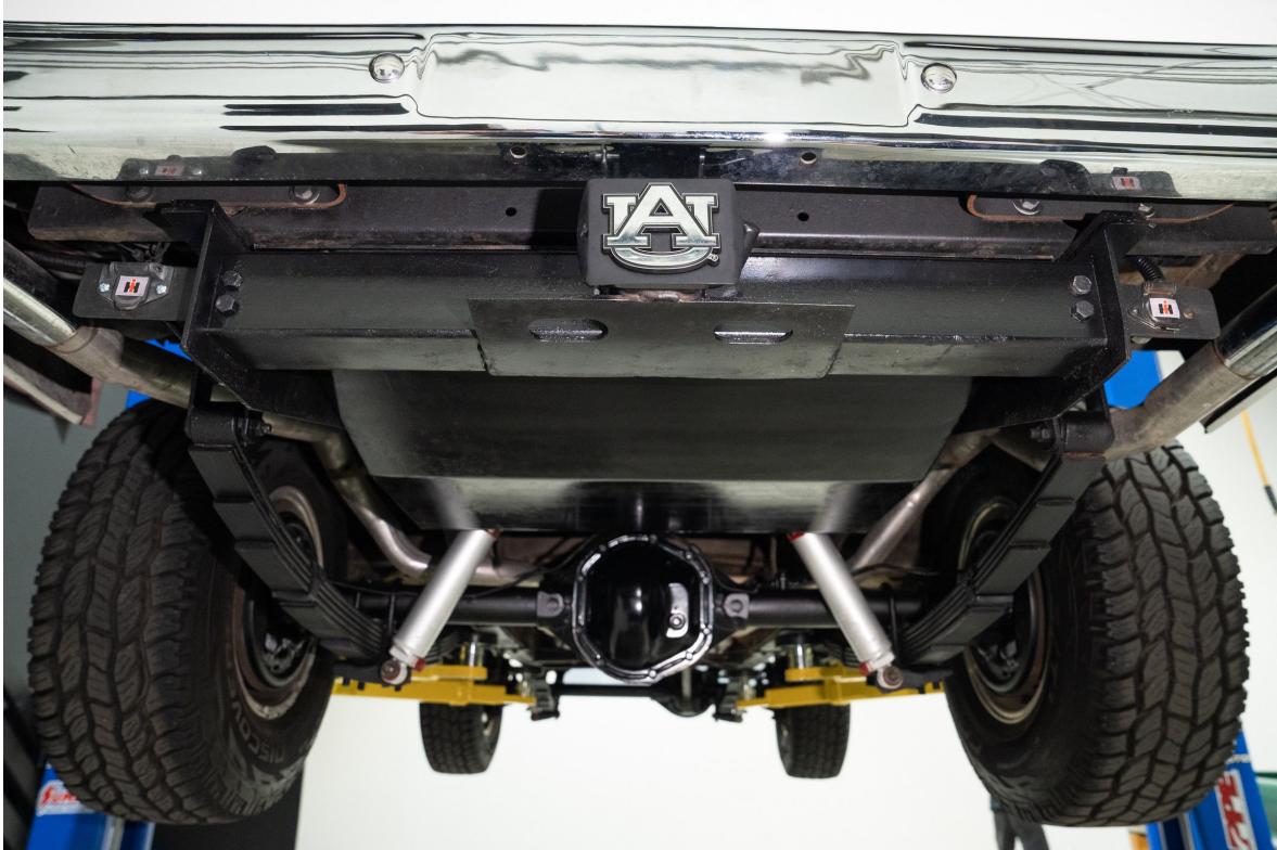
Rear view — painted skid plate, AU hitch cover, painted rear diff, IH frame stickers
