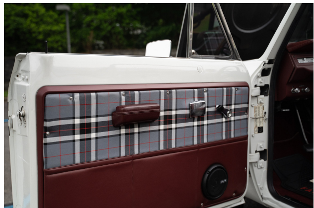
Door panel with tartan, marine vinyl, and Memphis 6.5" speaker
