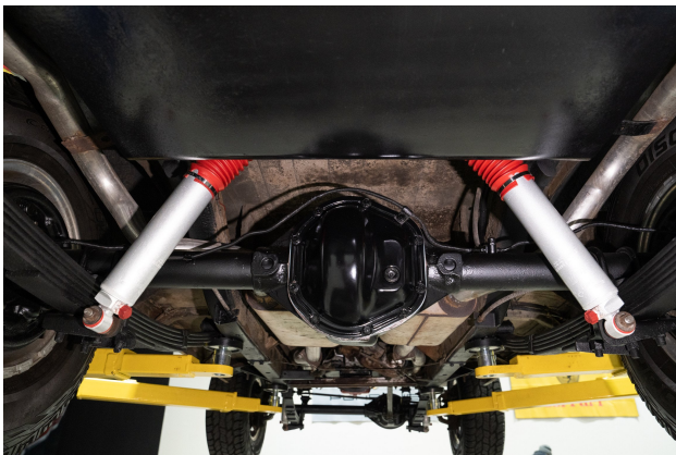
Rear Dana 44 with Rancho shocks and freshly painted diff cover
